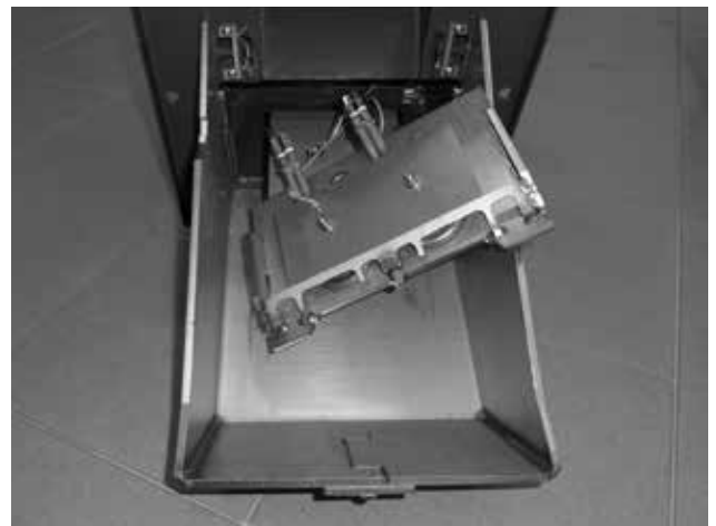
Fig. 4 - Disassembled plate with the ignition spirals
