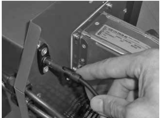
Fig. 6 - Photocell - be careful about its proper orientation - we recommend you to clean it at least once a year
