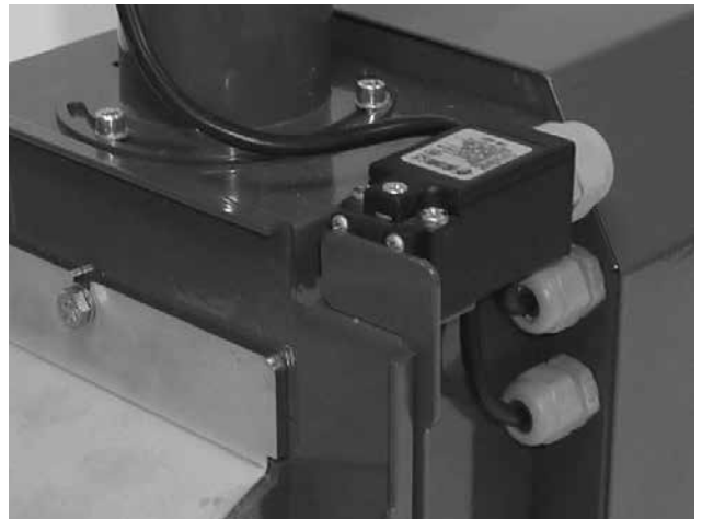
Fig. 8 - End switch with a special stop
