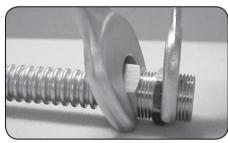
Tighten the double nipple to close up the existing trough to an evenly sealed position.
