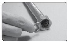
Insert the gasket and check for proper position of the lock ring.
