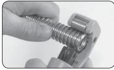
Cut the corrugated pipe at the desired place with a pipe cutter.
