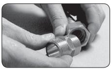
Turn in the appropriate fitting into the connecting nut (for example: fitting with external thread x compression fitting).
