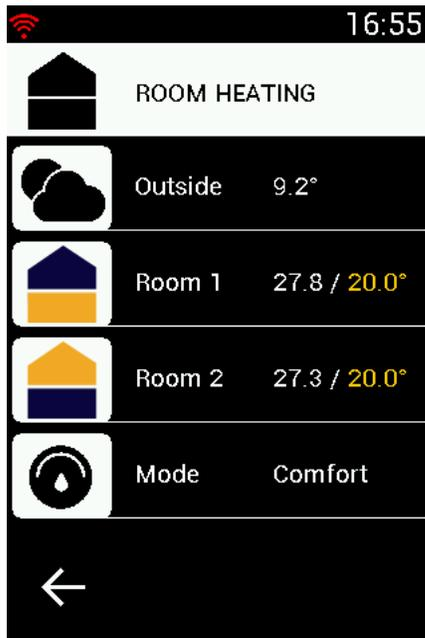
Room heating can be separately controlled if room sensors are used. In that case, the flow temperature of the heating circuits will depend of the room temperature desired.
