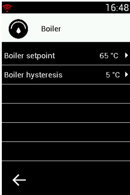
Under the option "Boiler" you can change the boilers setpoint and hysteresis, that are used in controlling the boilers electronic thermostat. The boilers thermostat will be turned on when the temperature of the boiler has dropped below setpoint - hysteresis level and turned off, when the temperature has risen above setpoint + hysteresis.
