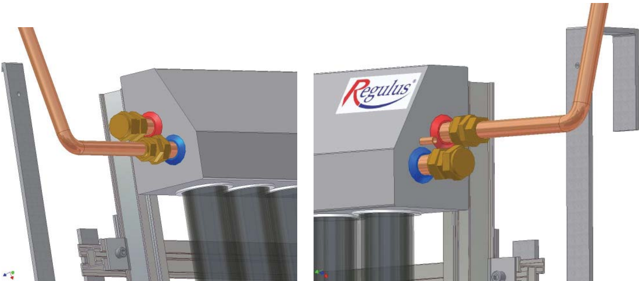
Fig. 25: Collector connecting (position of the inlet and outlet pipes and plugs)
