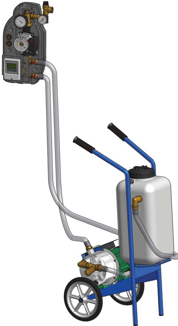
Fig. 34: Filling a solar system
