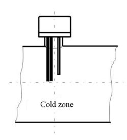
The unit built in too high and in reversed position (the protective guard is up).
