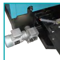
Gearmotor of automatic ash removal system
