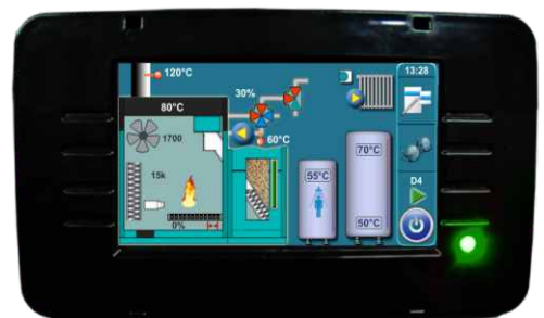
Multifunctional control with a touch screen display.
