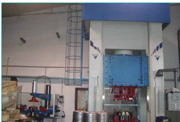
Forming of metal sheet with hydraulic presses
