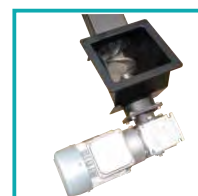
Connection of the burner with the tank feeder
