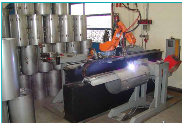
Robotic welding of stainless steel water heaters
