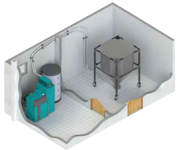
Example: Vacuum suction system by screw feeder from a storage room
