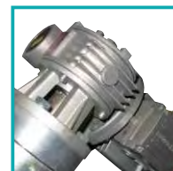
Motor with a gearbox of the pellet feeder
