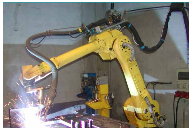
Robotic welding of the boilers
