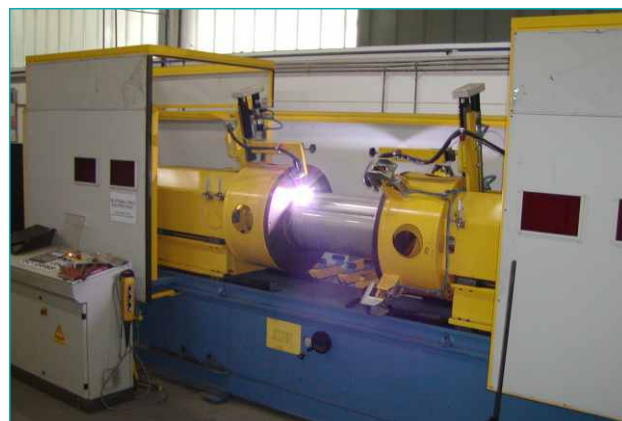
Automated welding of stainless steel water heaters
