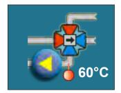
Motor device is opening the valve
