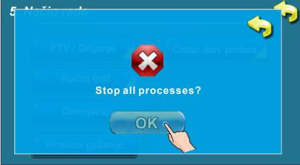
IMPORTANT! To be able to stop all processes, you must first turn off the boiler in the usual way by pressing on and then STOP.
