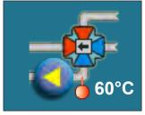
Motor device is closing the valve
