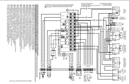
15. Electric wiring diagram for the boilers D20P, D30P, D40P, D50P with an extraction fan, modele 2012 with 6-pin connector and module AD02 - to control extraction fan of the boiler from burner control unit AC07X (R)
