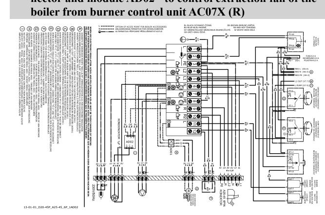
16. Wiring diagram connection of the boilers D20P, D30P, D40P, D50P with extraction fan, model 2012 with 6-pin connector and two modules AD02 - to control extraction fan of the boiler and pump in the boiler circuit from burner control unit AC07X (R and R2)
