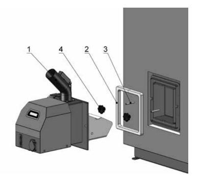
1 - pellet burner ATMOS A252 - Sealing cord 18x32 mm - small (code: S0165)
