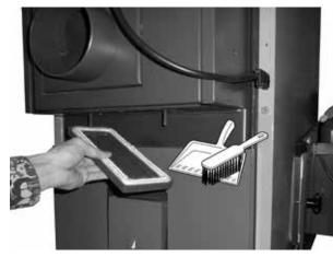
Sample cleaning of the smoke duct at the back side of the boiler
