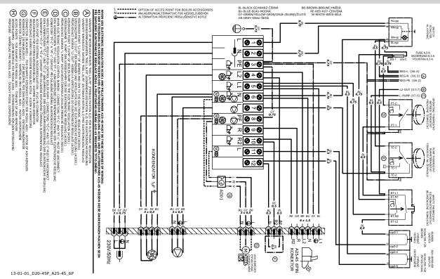
14. Electric wiring diagram for the boiler D15P without an extraction fan with a 6-pin connector and module AD02 to control pump in boiler circuit from burner control unit AC07X (R)
