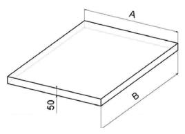
We recommend providing a concrete (metal) base under the boiler.
