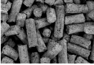
Poor-quality wooden pellets – dark with bark (with black dots)
