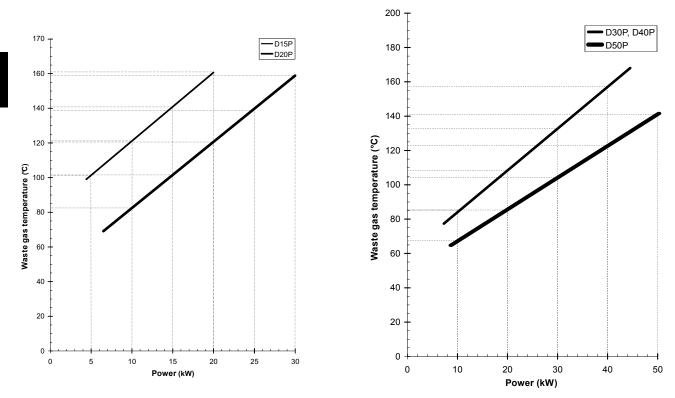
Relation of waste gas temperatur to boiler (burner) output when burning pellets
