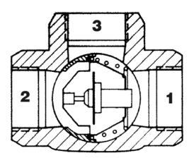
Thermoregulatory valve type TV 60 °C (65, 72, 78 °C) is used with solid fuel boilers. When the boiler water temperature reaches + 60 °C, the thermoregulatory valve opens and fluid from the building heating circuit (2) enters the boiler circuit (3  $\rightarrow$ 1). Inlets 1 and 3 always remain open. This ensures that the minimum temperature of the water returning to the boiler is maintained. If need be, a thermoregulatory valve set to a higher temperature (E.g. 72 °C) may be used.
