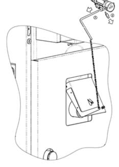
Disassemble the lever /1/ and coupler /2/ and screw the regulator into the boiler.
