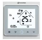
Voltage/Frequency: 230 V AC / 50 - 60 Hz Maximum current: 5A Operating temperature range: 0 - 45°C Regulation range: 5°C - 35°C Regulation accuracy: ±0,5°C External temperature sensor: NTC 10K Communication: R5485 Dimensions: 86 × 86 × 13,3 mm Weight: 270 g Degree of protection (housing): IP 20 Degree of protection (external sensor): IP 68
